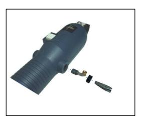
① Always remove the power cord from the outlet (socket) before replacing the brush. Remove the brush cap with a flat-bladed screwdriver and replace it with a new brush. The minus (—) side of the brush wears out more than the plus (+) side. Replace with a new brush before the brush length falls to 5mm or less.
